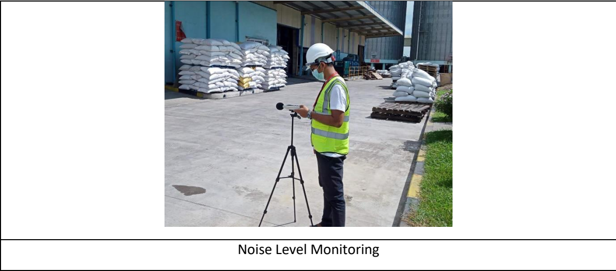
Figure 1-9 Noise Level Measurement in the Factory
